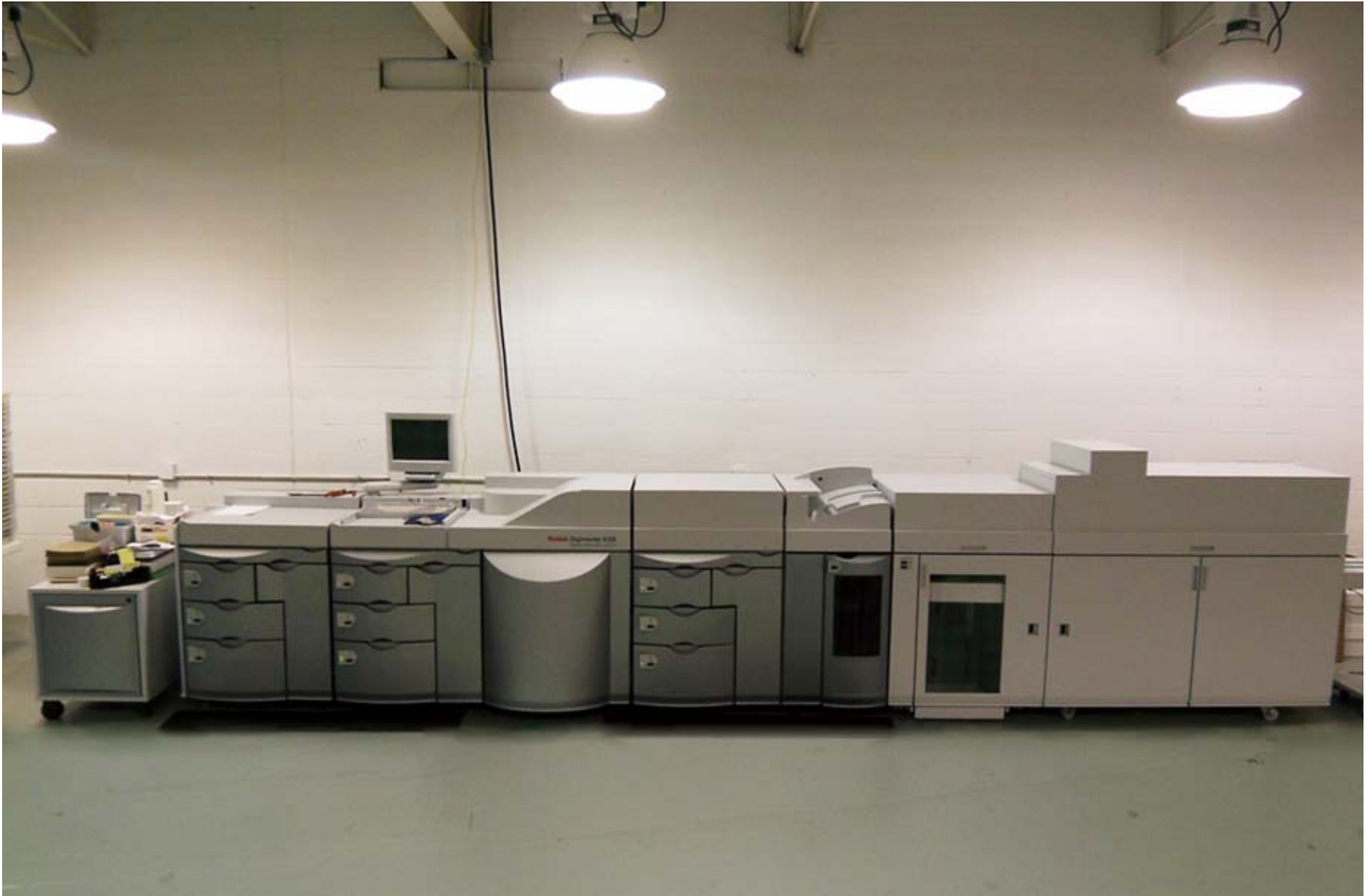
FormStore's Kodak Digimaster with Interposer and C.P. Bourg Saddle Stitch Digital Print & Direct Mail Power
